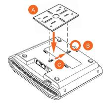
4 (Optional) Attach a customer-supplied padlock through the integral AP retainer tab (B in <u>Figure 3</u>) to fasten the AP to the secure mounting bracket studs.
